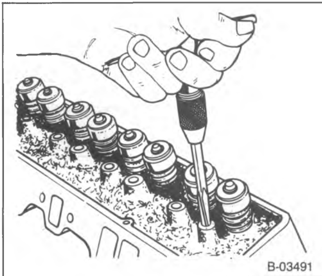
Figure 13—Reaming the Rocker Arm Stud Bore (Typical)
