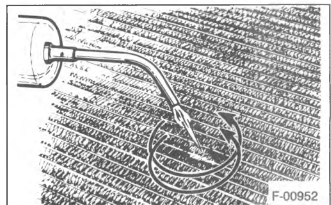
Figure 31—Heating the Repair Area
