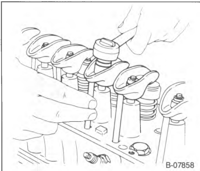
Figure 4—Adjusting The Valves
