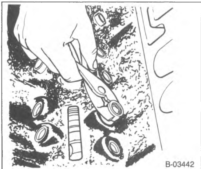
Figure 7—Removing the Valve Lifter
